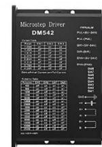
Gambar 2. Driver Motor Stepper
