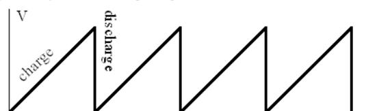
Gambar 12 Signal output transistor TR<sub>2</sub>
